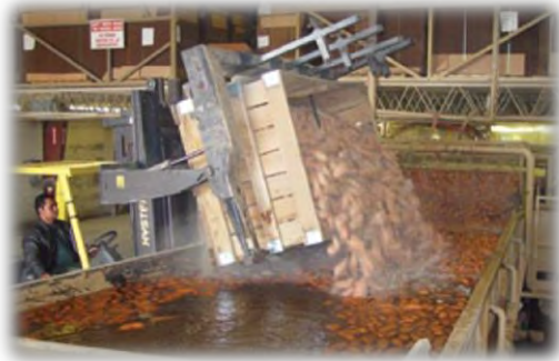
Pouring sweetpotato roots into water using a fork-lift mounted bin rotator device
