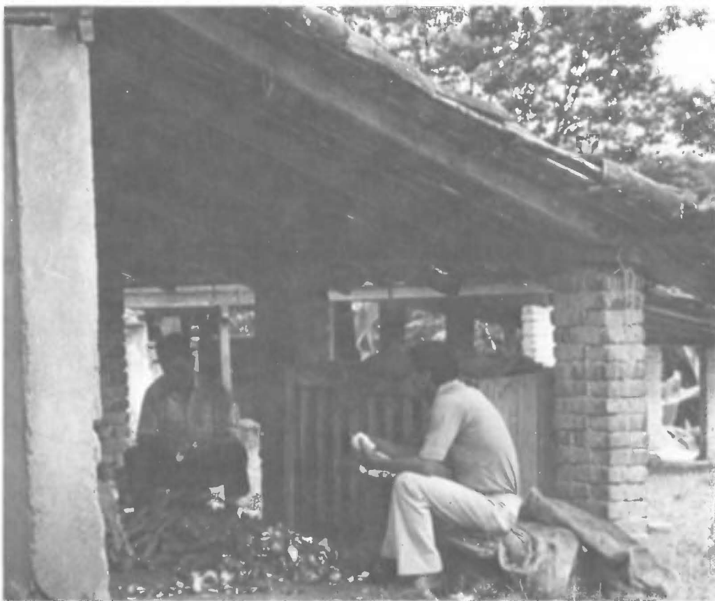
Fig. 3. In this small-scale starch factory, the roots are peeled by hand but not washed beforehand. The ash content, therefore, is likely to be high.
