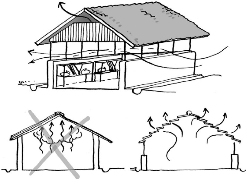
Figure 19: Roof construction in relation to ventilation
