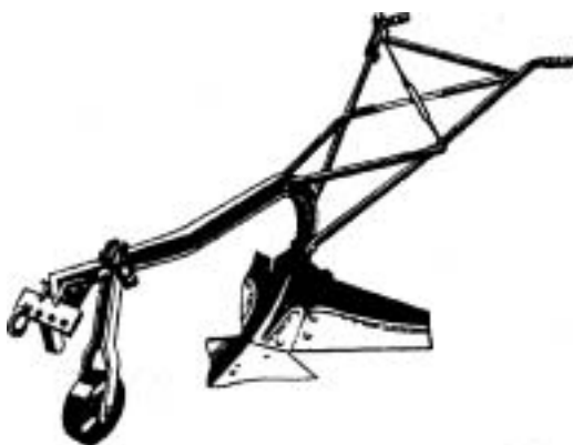
Figure 39: "Inkunki" high wing ridger, manufactured in Zimbabwe.
