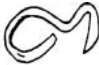
Figure 8: A hoof pick can be easily made by bending a piece of round steel into the desired shape with one end flat and pointed.
