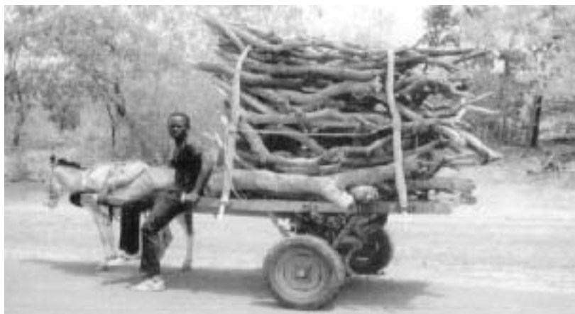
Figure 30: Two-wheel donkey cart in Mali. Provided the load is well balanced, donkeys can pull impressive loads along flat roads.
