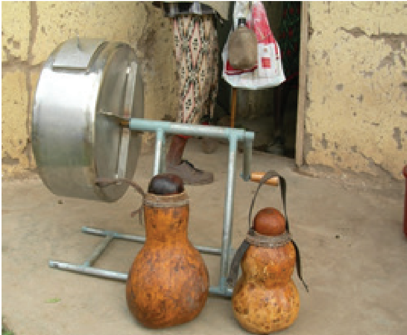
Figure 3. Improved aluminium manual butter churn.
