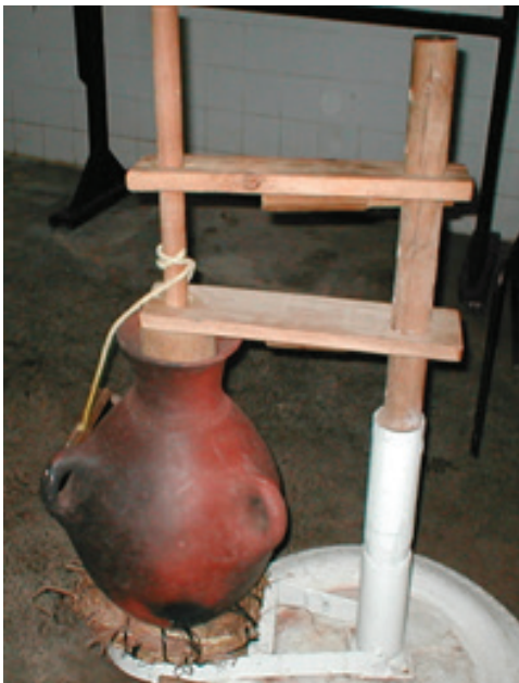
Figure 2. Traditional clay pot butter churner with the ILCA developed internal agitator with paddle blades.
