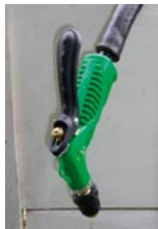
Fig. 3.3 Spray gun, adjustable to give a single jet or a wide spray. (Photo: P. Fellows)
