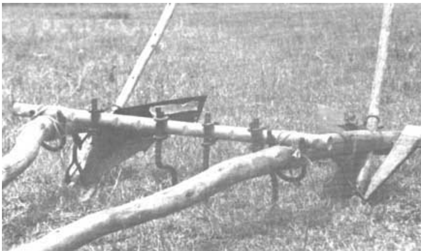
Figure 8. Tine harrow fixed on the cross-beam of the broadbed maker.
