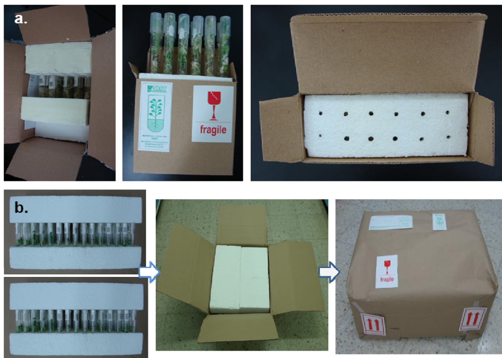
Figure 3. Packing system for in vitro seedlings in styrofoam racks: a) Packing system for individual racks, and b) Packing for two racks, in both cases racks are protected by styrofoam structures.
