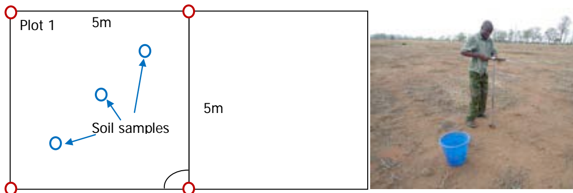
Figure 5. Location of the soil sampling points within a plot and a field technician on the job. A bucket/basin is an important field tool for mixing soils to get a representative sample.
