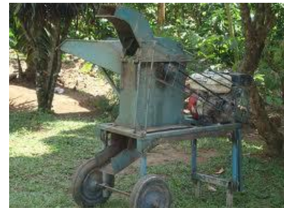
Figure 2: An example of a pulveriser used by small scale farmers. Source: EADD web site
