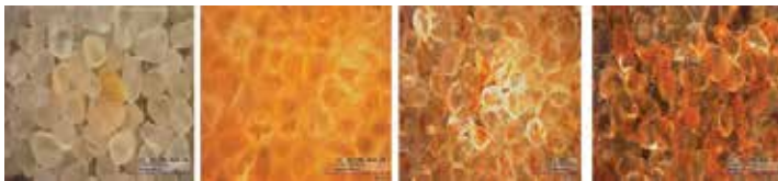
Figure 3. Microscope image of infiltration measurement showing the sand column at the start of the measurement, 30 minutes of soil solution application, 1 hr application and 2 hours after the second soil solution infiltration on the previous sand column, respectively.
