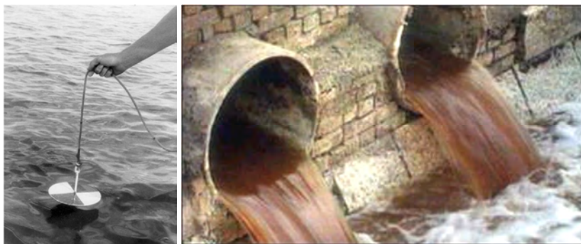
Figure 3-6: A Secchi disk is used to measure water clarity. Discharge of effluent into natural waterways can reduce water clarity.
