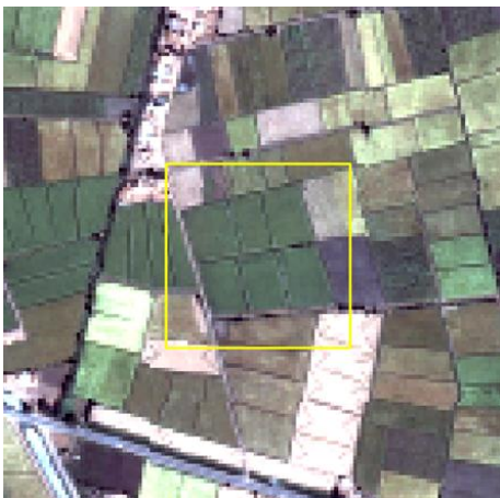
Figure 2: A high-resolution 5 m IKONOS image (of a different year) with the selected 240 m coarse-resolution image (yellow box) superimposed, to illustrate how the 240 m pixel size relates to individual field sizes.
