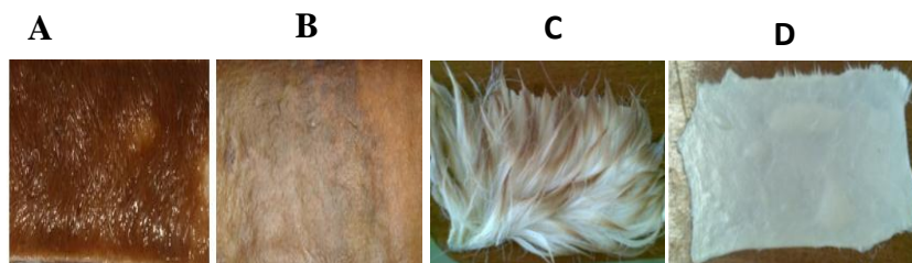
Fig. 5: Enzymatic dehairing of cow hide and sheep skin. A) Cow hide treated with buffer alone; B) Cow hide treated with alkaline protease C-45 pH 10 buffer; C) sheep skin treated with buffer alone; D) Sheep skin treated with alkaline protease R-11
