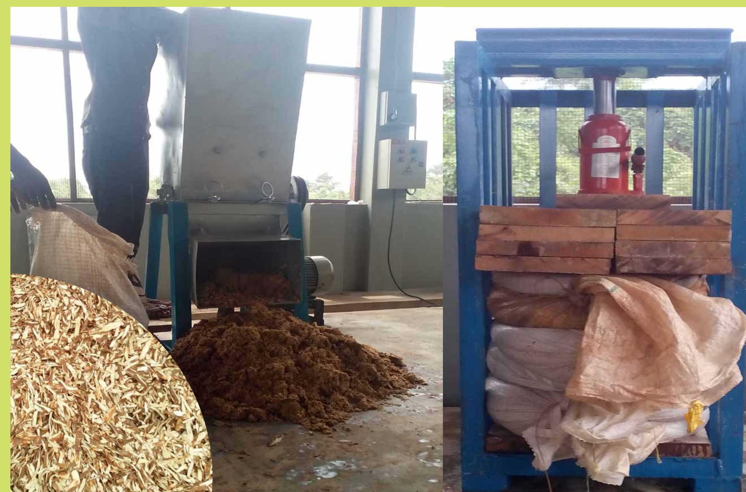
Figure 3. Grating and dewatering cassava peels for sun drying (ongoing technical innovation).
