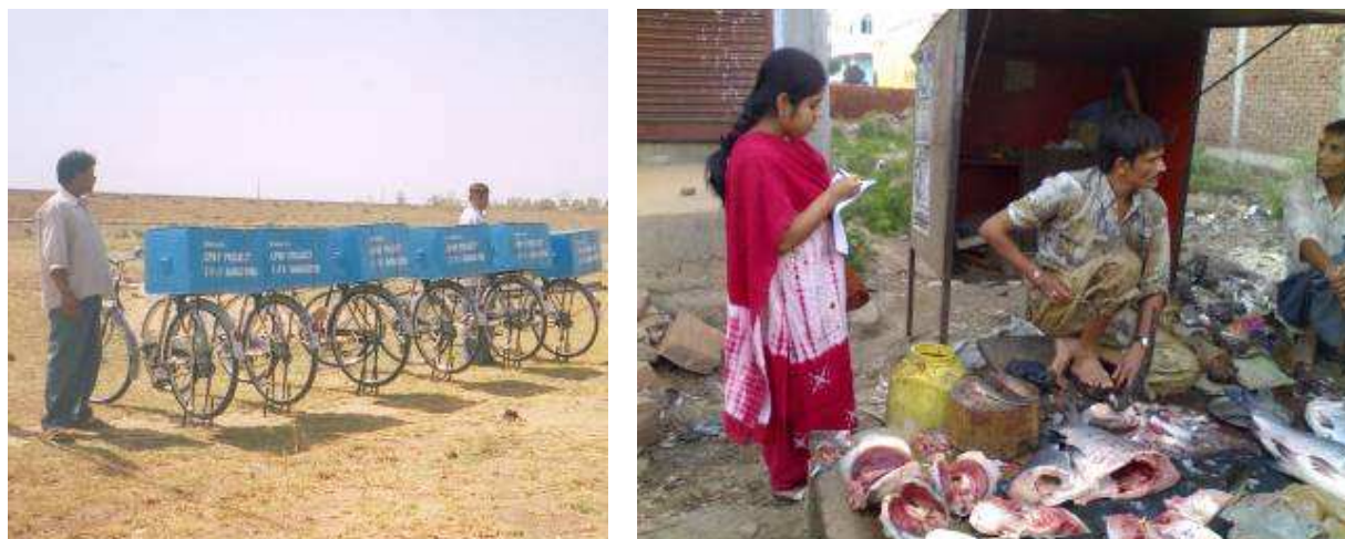
Photos 3.3. Left: bicycles fitted with iceboxes to improve quality of fish during transportation. Right: Market survey.
