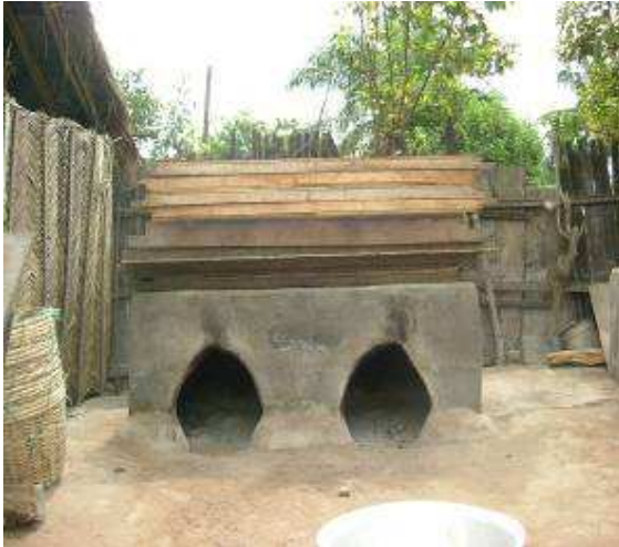
a. Chokor Smoker with a pile of trays to contain fish for smoking. Openings for fuel wood directly under fish.
