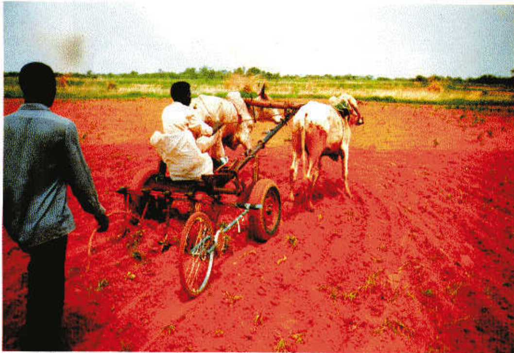
Plate 2. A pair of oxen pulling a Nikart tool bar at the ICRISAT Sahelian Center in Niger with an ergometer attached to measure work output.
