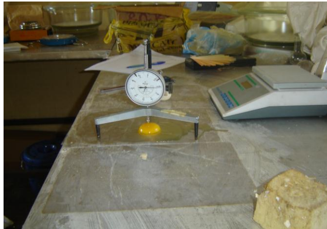
Tripod micrometer used for measuring yolk height and albumen height
