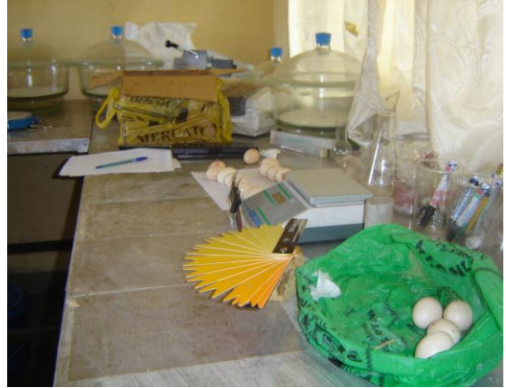
Yolk color measuring fan graded from 1 to 15
