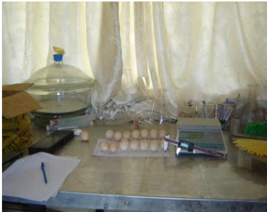
Caliper, used for calculating egg shape index and shell thickness
