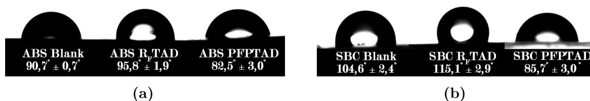
Figure IV.1: Static contact angles of the blank (left), R F TAD modified (middle) and PFPTAD modified (right) polymers, i.e. acrylonitrile butadiene styrene terpolymer (ABS, (a)) and styrene-butadiene copolymer (SBC, (b)).
