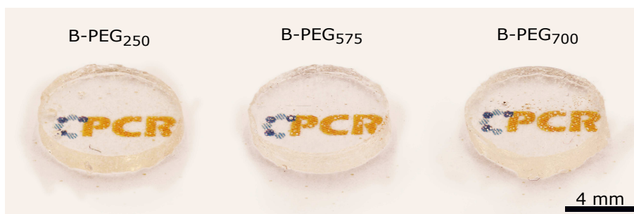
Figure VIII.3: Pictures of the PDMS- l -PEG co-networks (Table VIII.1).
