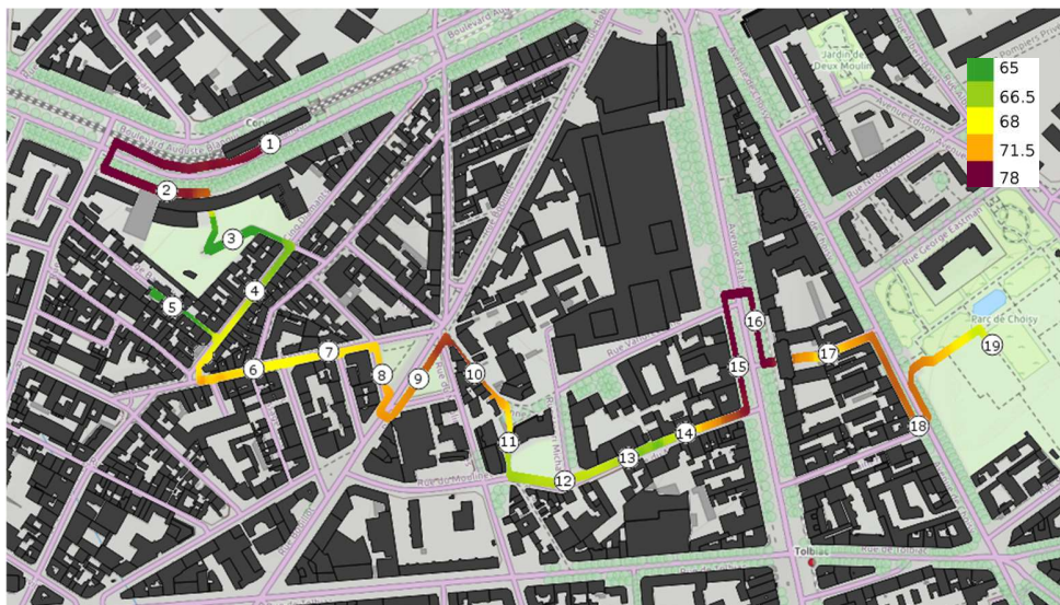
Figure 1 Sound map of the studied path, interpolated from mobile measurements ( L_{eq} - dB). The points 1 to 19 correspond to the different assessment locations.
