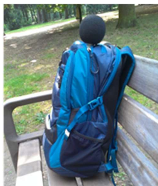
Figure 2 Backpacked sound measurement station.
