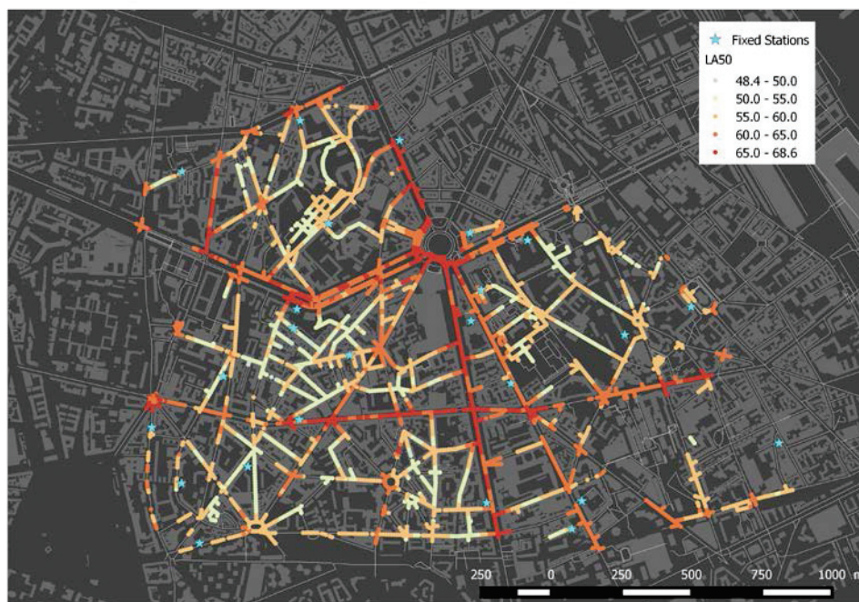
Figure 1 – Reference sound map of the \hat{L}_{A50,[10-12h,14-16h]} and location of the 23 fixed stations (stars).
