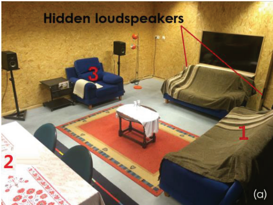
Figure 1 – The mock up living room with hidden environmental noise loudspeakers indicated next to the mock-up window.
