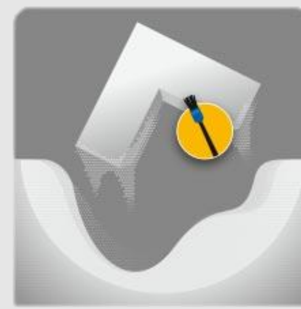
Afterwards, the loose powder is removed and the product is cleaned
