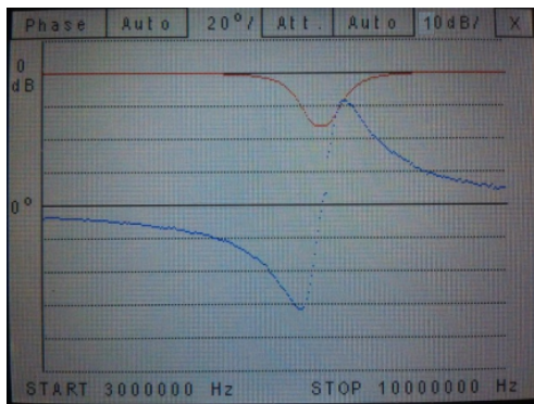
Fig. 6: 6 MHz notch filter with proposed design.
