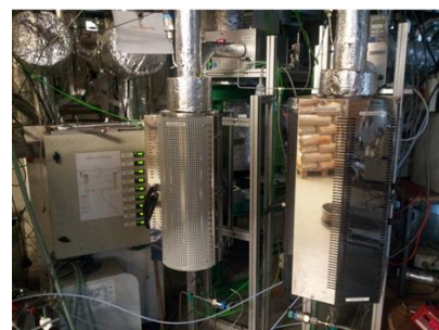
Figure 1. (left) \text{CH}_4 concentration in gas during dual bed duration test at 900^\circ\text{C} , GHSV \sim 5000 \text{ h}^{-1} ; (right) MILENA gasifier and catalyst reactors.
