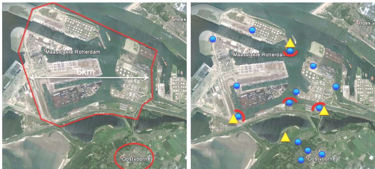
Figure 1 – Left: indication of the size of the industrial area (IA) and the distance to the residential area (RA). Right: Locations of the microphones, arrays, and meteorological masts.
