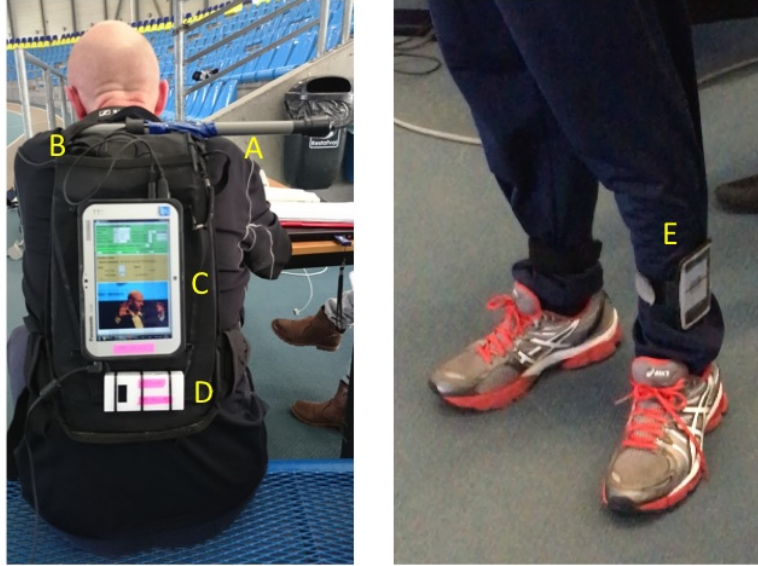
Figure 1.2: The equipment mounted on the backback consisting of (A) a sonar distance sensor; (B) headphones, (C) 7" tablet, (D) Wi-Fi router, and attached to the ankles (E) iPods.
