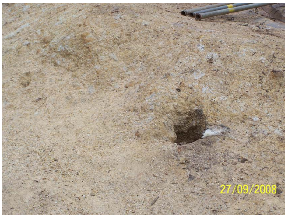
Figure VII.41. Photo of aquifer materials excavated in recently constructed wells showing a mixture of kaolinite and muscovite minerals
