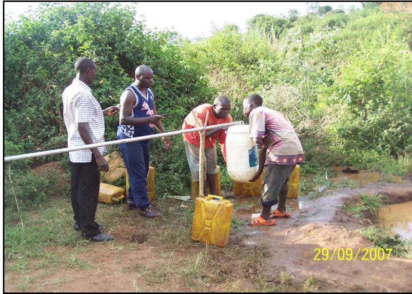
Figure IV.4. Discharge measurement during the pumping test
