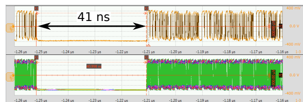
Fig. 4: packet with a long gap (41 ns).
