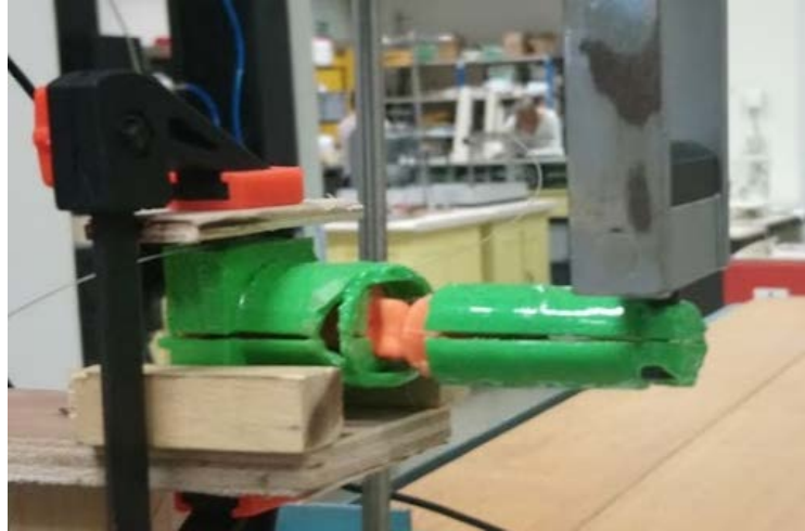
Figure 2. Test setup: artificial finger in INSTRON tensile tester
