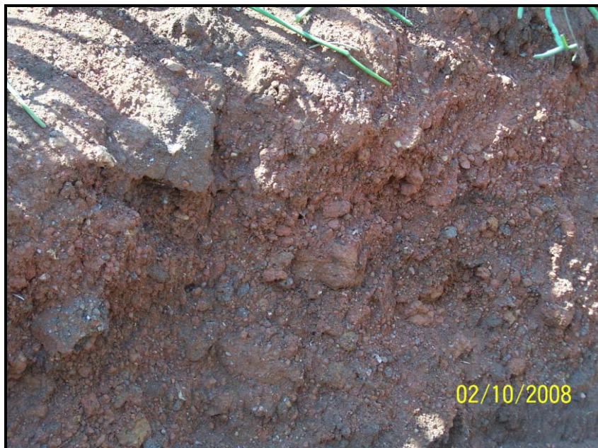
Figure IV.12. Geological materials excavated at the bottom of the well in Kiruhura I-Kiyanza (Nr. 23) showing that the aquifer is mainly made up of a mixture of reddish sand, lateritic gravel and rock fragments.
