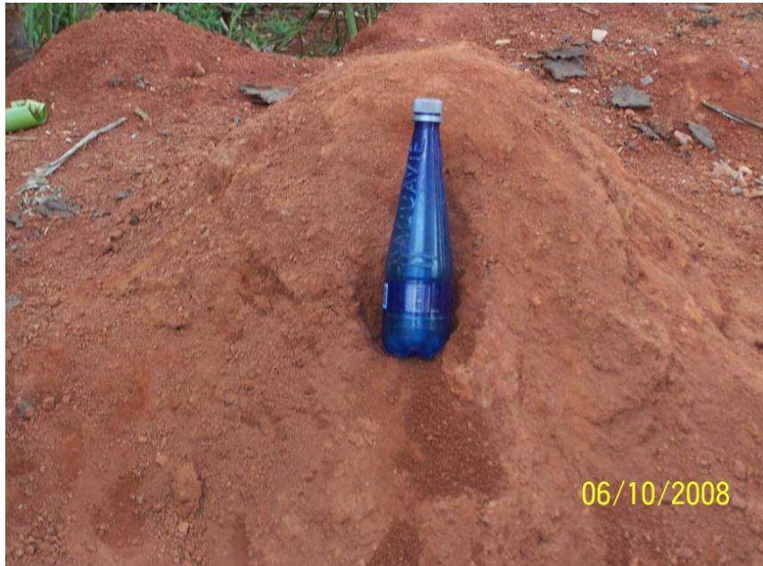
Figure IV.11. Geological materials excavated at the bottom of the well in Kiruhura II-Muramba (Nr. 22) showing that the aquifer is made up of a mixture of reddish clay, sand and lateritic gravel.
