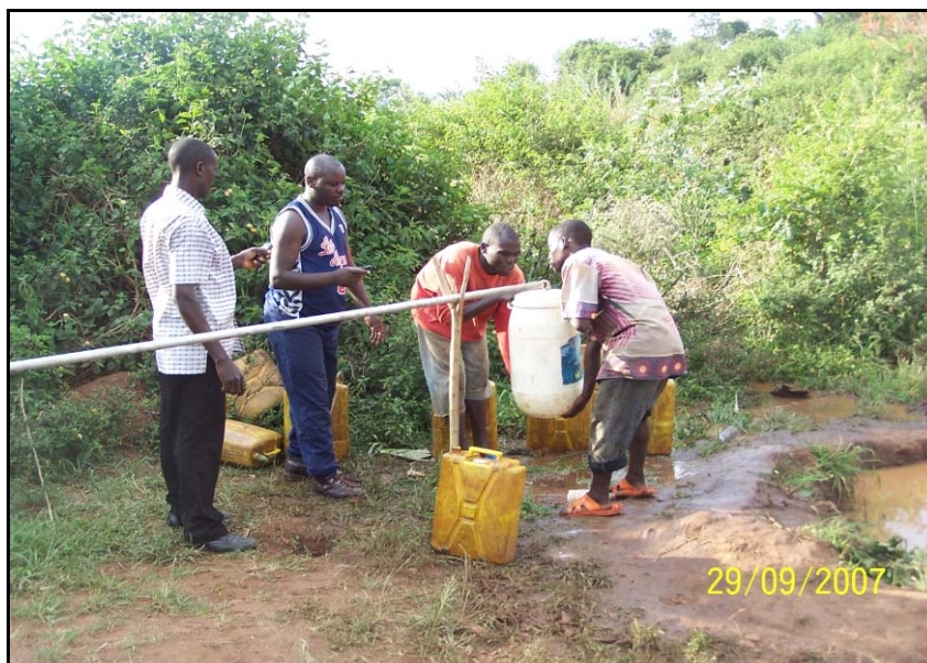
Figure IV.4. Discharge measurement during the pumping test
