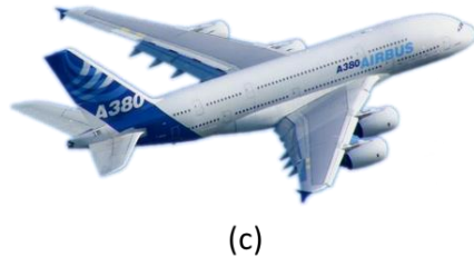
Figure 2 – Straw/clay composite bricks found behind the plaster of a house in Nicosia, Cyprus (a), the first ever produced 1953 Corvette C1 (b) and the Airbus A380 which has about 50% of its structural parts made from composites (c).
