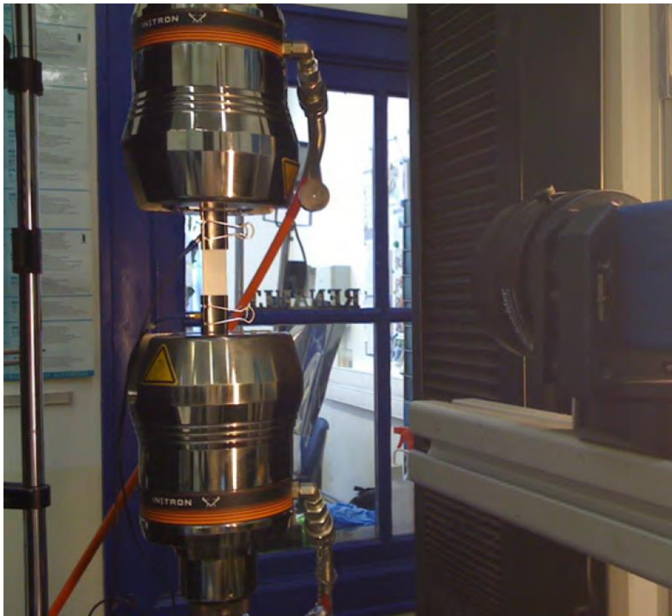
Figure 10: Tensile test with the assistance of acoustic emission (AE) and strain mapping.
