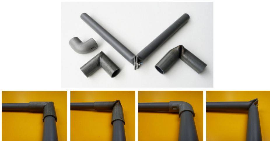
Figure 5.12. Alternative ways to create the same 90° joint, as reported in the Modular vegetable protection cage project
