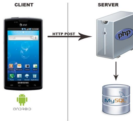
Figure 2.18 Client - Server Architecture in Android Platform (Rahman, 2011)
