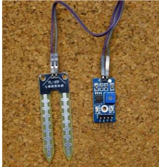
Figure 2.0.5: YL-69 Moisture Sensor (Probes) Source: Guide for Soil Moisture Sensor YL-69 or HL-69 with Arduino, 2016
