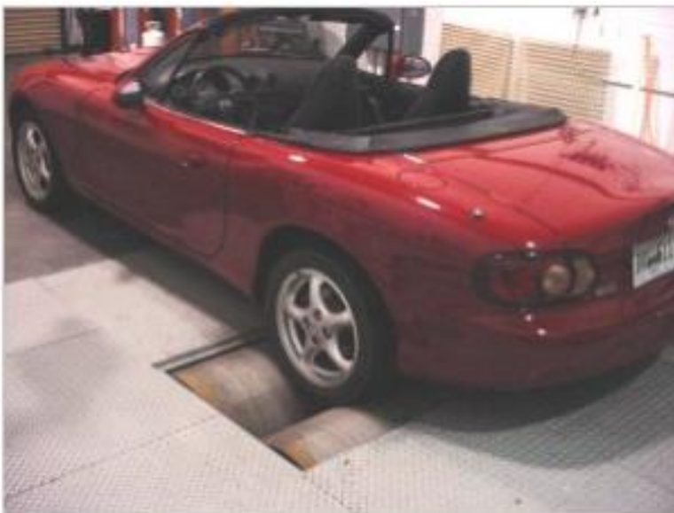
Figure 2.4 A Vehicle on a dynamometer during a lab test. (Adapted from fueleconomy.gov, 2016)
