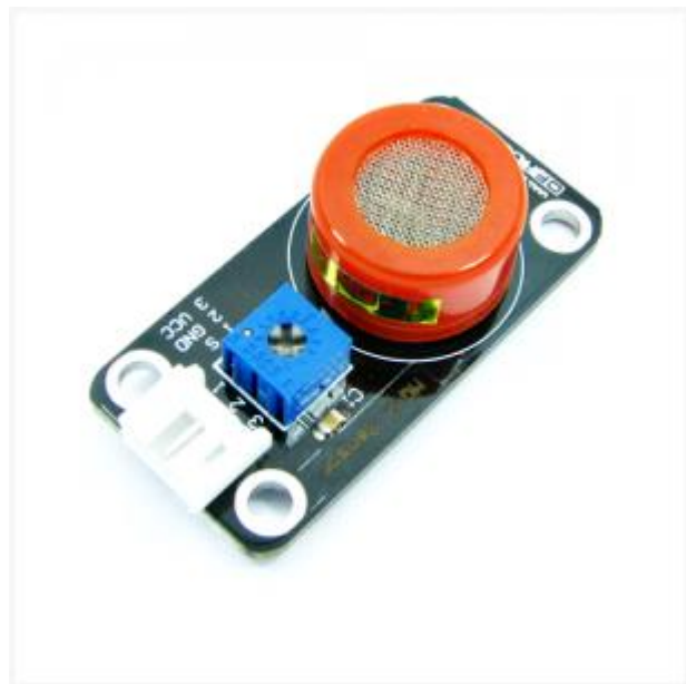
Figure 2.10 MQ-7 Carbon Monoxide Sensor. (Adapted from store.nerokas.co.ke, 2016)
