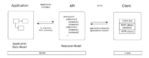
Figure 2.1: API Components (Adapted from Geert, 2017).
