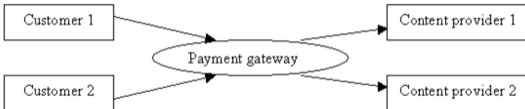
Figure 2.6: Architecture of a collaborative micropayment system (Pocatiu & Ciurea, 2009)
