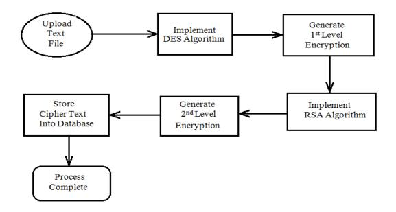
Figure 2: 6: Block Diagram of Multilevel Encryption (Khan & Tuteja, 2015).
