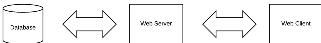
Figure 5.1: Application architecture of the proposed recommender system
