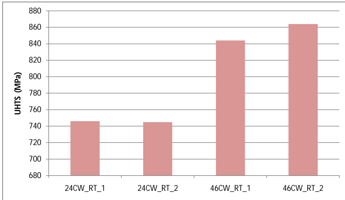
Figure 13. Ultimate hoop tensile strength (UHTS) vs. CW for 15-15 Ti at room temperature
