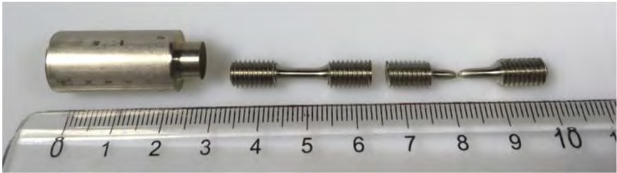
Figure 24. 20%CW specimen (BK), the percentage elongation after fracture A_t=43\% and the reduction of Area Z=81\% .
