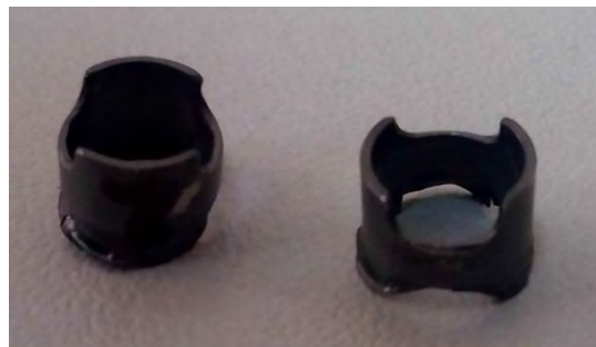
Figure 15. The ring tension specimens covered with the colloidal graphite.
