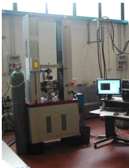
Fig. 9: Metrocom E50 Machine (left); flattened tubes after testing (right)
