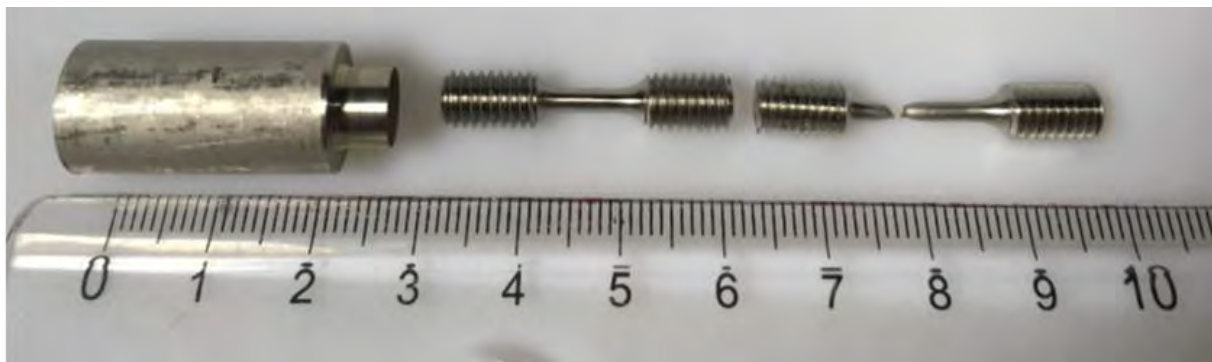
Figure 25. Annealed specimen (BL), the percentage elongation after fracture A_t=69\% and the reduction of Area Z=73\% .
