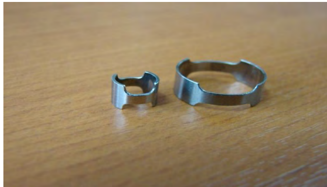
Figure 6. The Ti-Ti15 (24%CW) specimen vs. Zy-4 specimen for ring tension test
