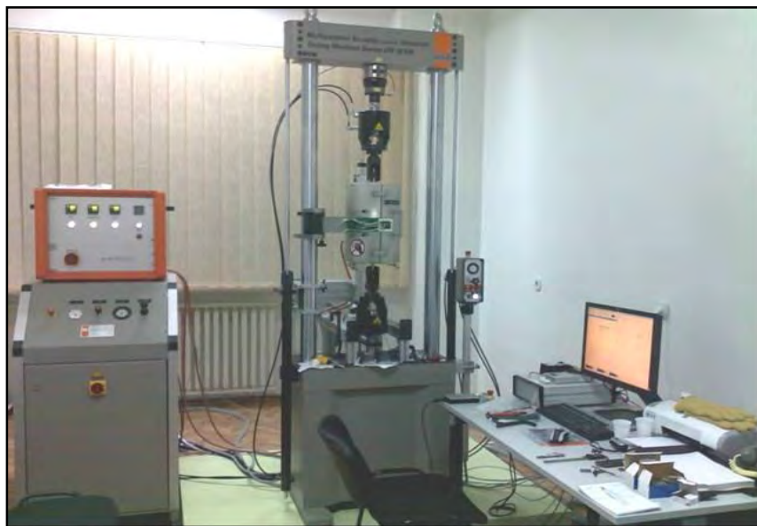
Figure 8. The testing facilities (Walter Bai Testing System and acquisition system)
