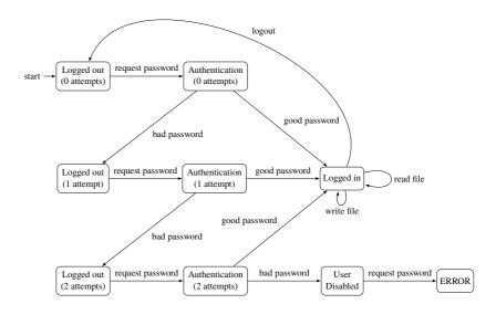
Fig. 1. An automaton-based specification
