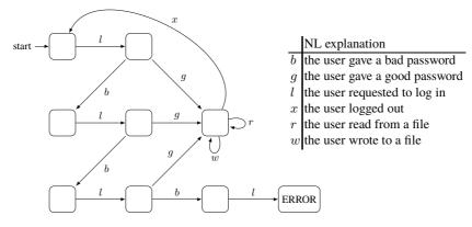
Fig. 2. The specification augmented with NL explanations
