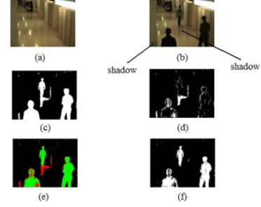
Fig. 2. Shadow detection and removal process (a) Background model, (b) Current Frame (c) Output from the Motion Detection module, (d) Shadow Detection, (e) foreground is shown in green while shadow is depicted in red and (f) Resulting frame with suppressed shadows.
