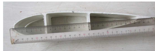
Figure 12 - Pultruded sample blade section.
