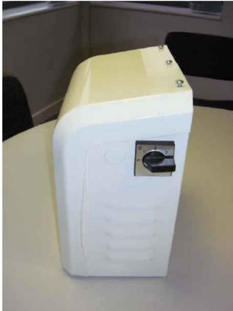
Figure 1: VO4Home unit showing the three voltage tapings.
