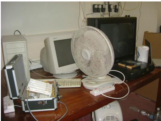
Figure 3: Actual test photo showing the PL lamps (in a case), desk fan, pc and monitor, TV and DVD player, the cfl lamp (behind TV) and the kettle at the far right. The fluorescent tubes can be seen behind the monitor.
