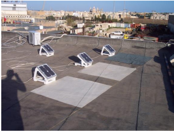
Figure 1: PV modules in front of paint, cement and waterproofing membrane, covering horizontal flat roof. The fourth module is the reference.
