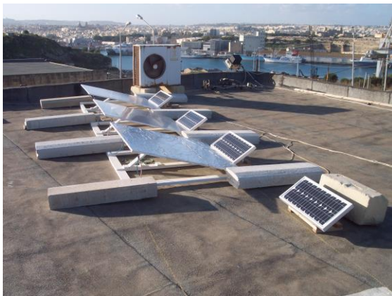
Figure 2: PV modules in front of three inclined reflectors covered with aluminium foil, aluminium sheet and white painted board. The module of the right was the reference module.
