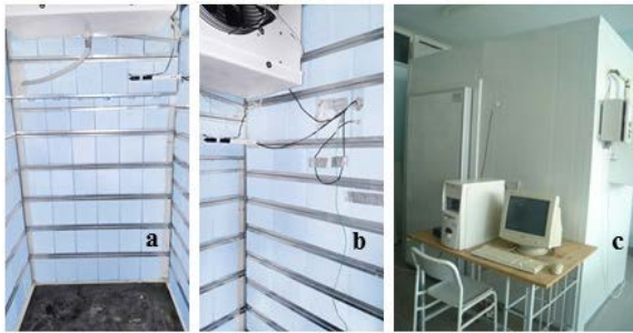
Figure 1: The cold store cabin: (a) inner view, (b) position of the sensors and (c) outer view
