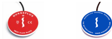
Figure 1: View of the Hukseflux HFPO1 heat flux sensors used to measure the heat flux through the building blocks being tested
