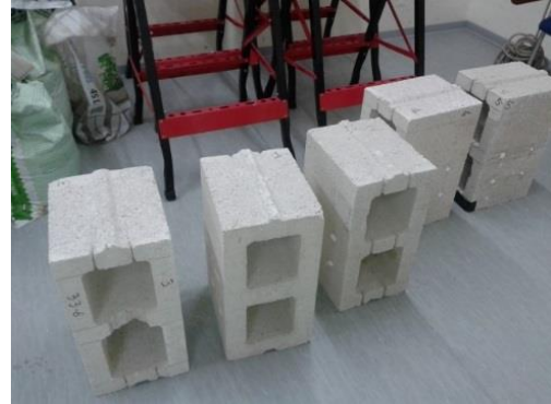
Figure 5: HCBs weighed and thermally tested ready to be taken for compression testing.
