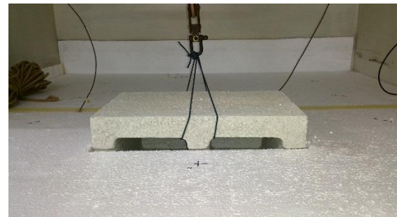
Figure 2: Individual HCBs placed within a cut-out of expanded polystyrene sheet, suspended in place through the use of a pulley system. (Hot box setup in the laboratory at the Institute for Sustainable Energy, University of Malta)
